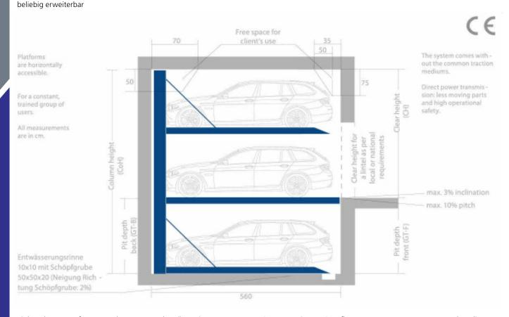
Pit length 555 cm, for 500 cm long cars. Further dimensions upon request. Concrete: min. 18, C25, floor evenness acc. to DIN 18202 Tab. 3, line 3. Load per parking space: max. 2.000 kg, wheel load: max. 500kg. Optional up to 2.300 kg or max. 2.600kg, wheel load max. 650kg.
