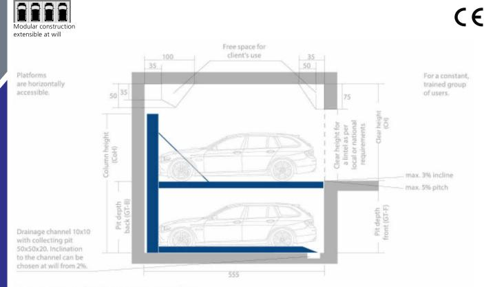
The system comes without the common traction mediums. Direct power transmission with lifting platforms directly welded to the lifting carriages less moving parts and high operational safety.
