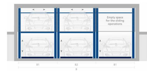
On the entrance level are sliding platforms with one empty space on the right (on the left: possible as an option). On the lower level the system is provided with lifting platforms. A lifting platform will be lifted to the empty space on the entrance level.
